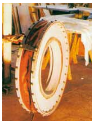
Tube-compensator for a low-fired calcination equipments
