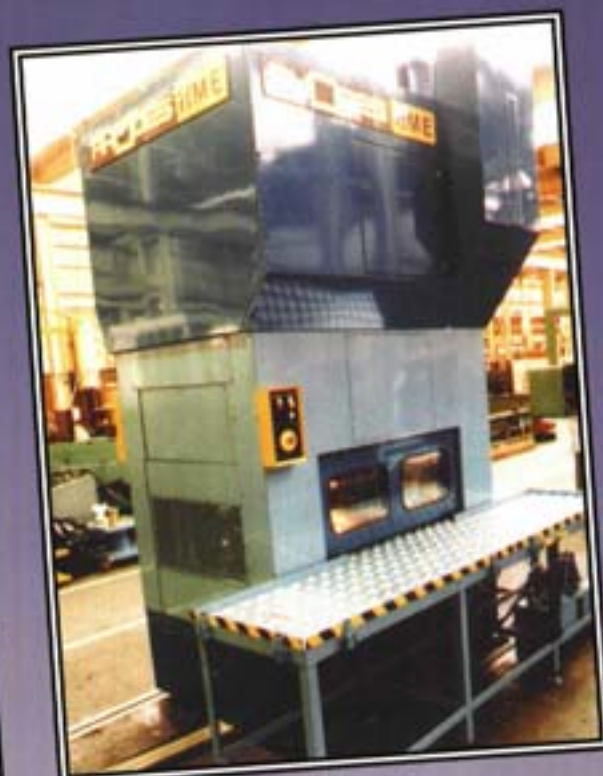
Die table for fast tool changes.
