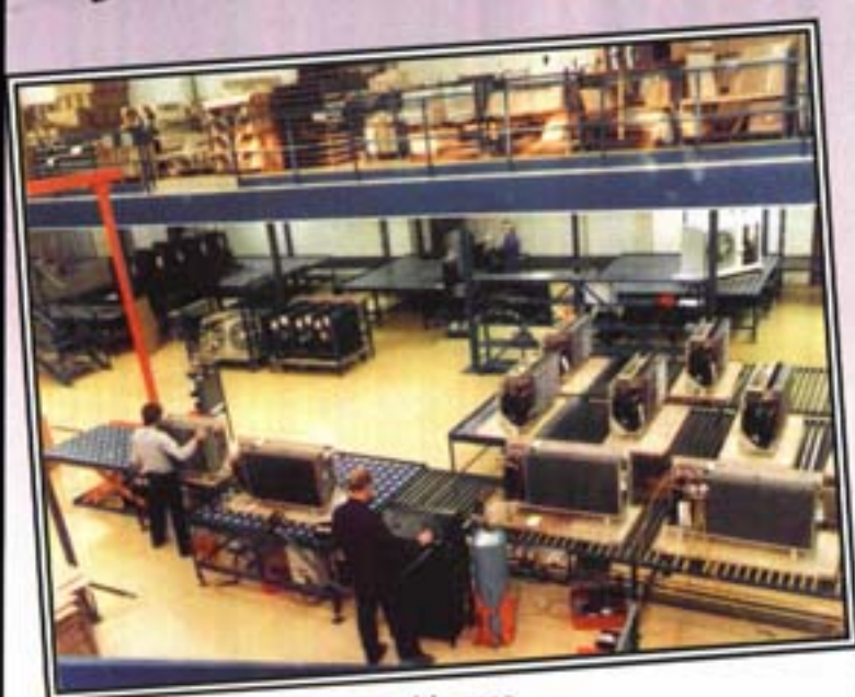
Tilting ball table used in conjunction with gravity racking.
